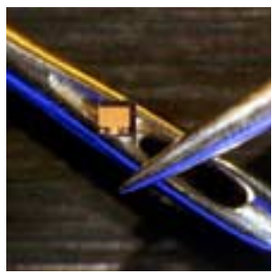
i. Diode laser chip: environmental monitoring, medical diagnosis, communication
