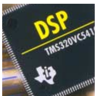
e. DSP chip: cellular telephony, controlled braking, network connection
