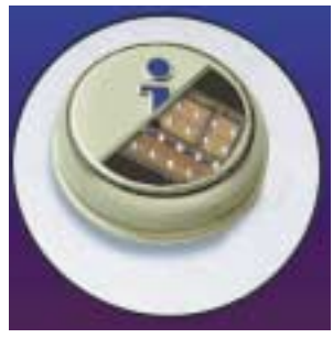
o. Ibutton chip: bar coding, delivery tracking, asset tagging, temperature sensing
