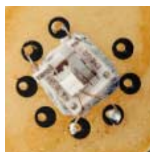
h. Hygrometer chip: measuring moisture
