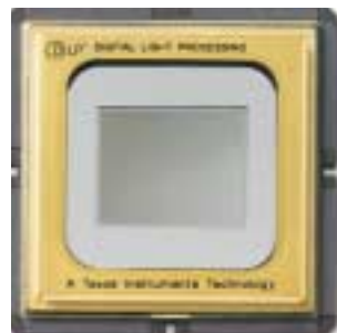
d. DLP chip: movie and video projection, photo finishing
